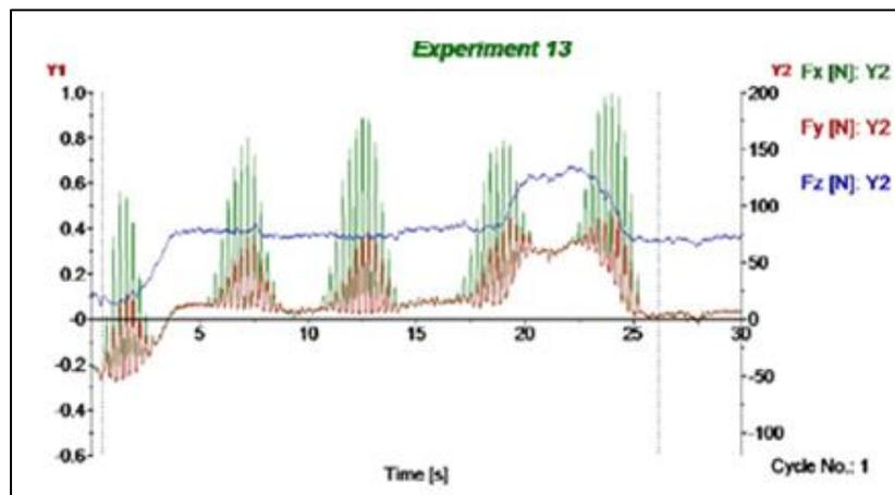
Fig. 6: Sample Graph of Cutting Forces
