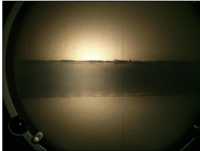
Fig. 8: Sample Delamination Profile
