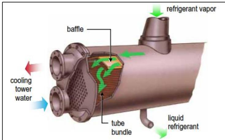
Fig. 2: Heat Exchanger type Condenser
