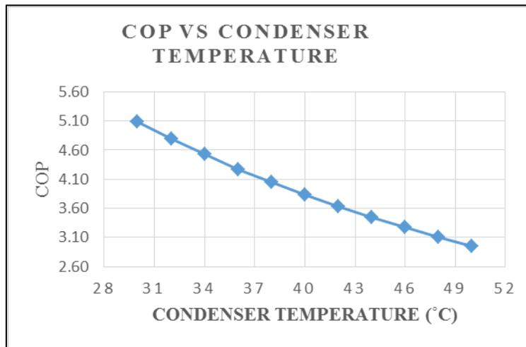
Fig. 9: COP Vs Condenser Temperature At Constant Evaporator Temperature
