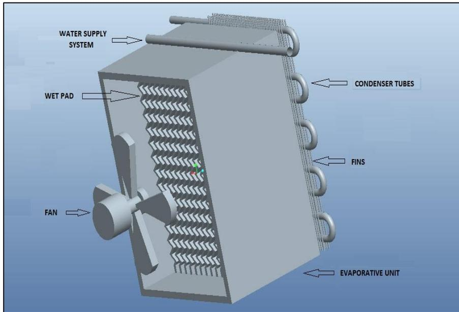
Fig. 4: Modified Air cum Evaporative Condensing Unit
