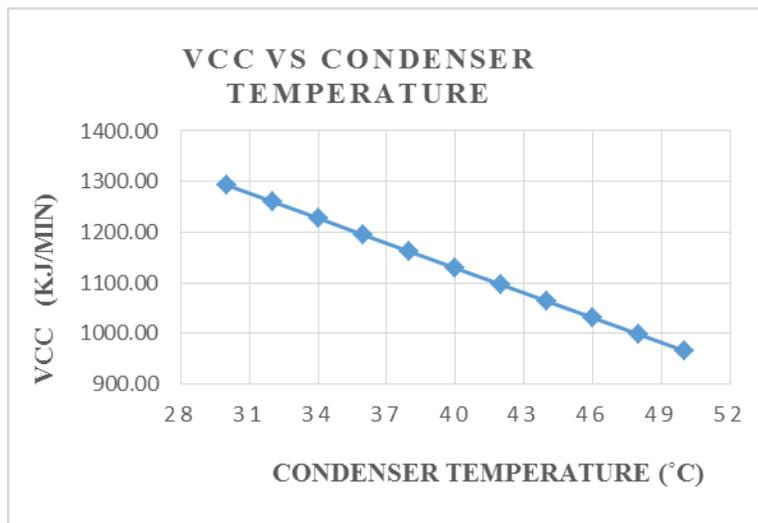
Fig. 8. VCC Vs Condenser Temperature at Constant Evaporator Temperature
