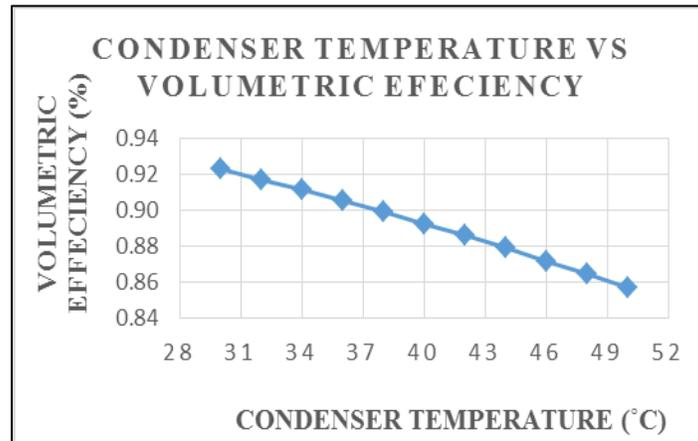
Fig. 6:  $\eta$ volumetric Vs Condenser Temperature At Constant Evaporator Temperature
