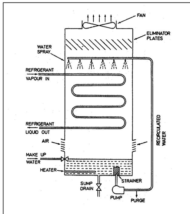
Fig. 3: Water Spray Type Condenser
