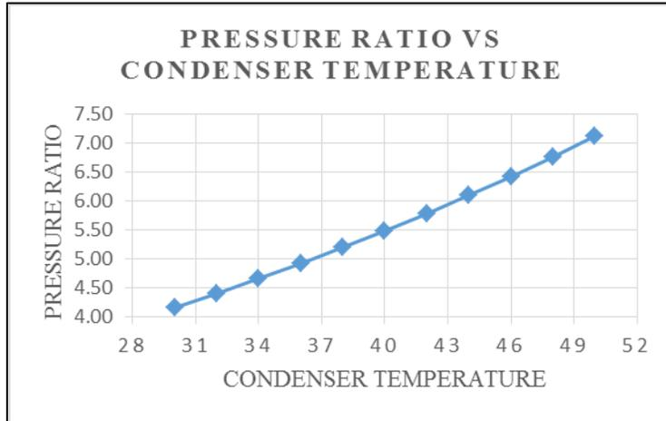
Fig. 5: Pressure Ratio Vs Condenser Temperature at Constant Evaporator Temperature
