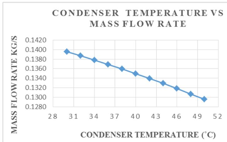
Fig. 7: Mass flow rate Vs Condenser Temperature At Constant Evaporator Temperature
