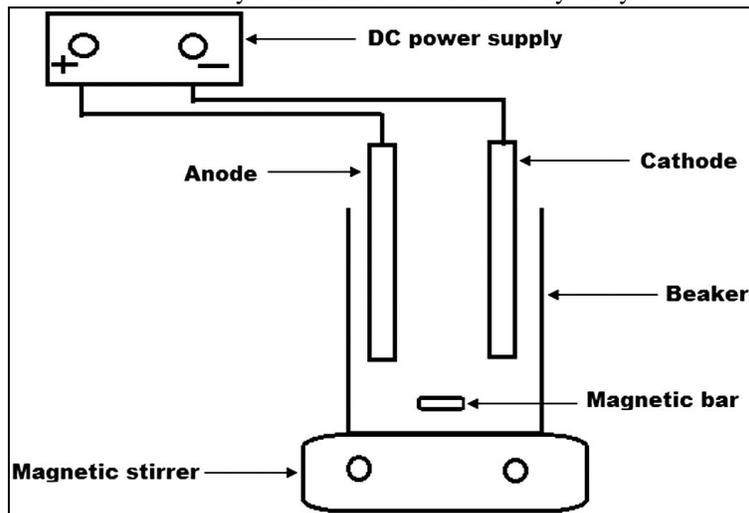
Fig. 1: Batch Mode Electrocoagulation Experimental Setup
