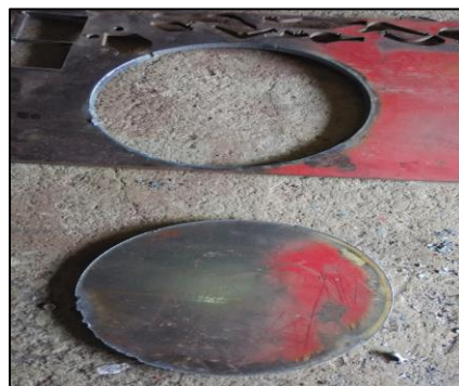
Fig. 7: Cutting Sample Of Thickness 16 Mm
