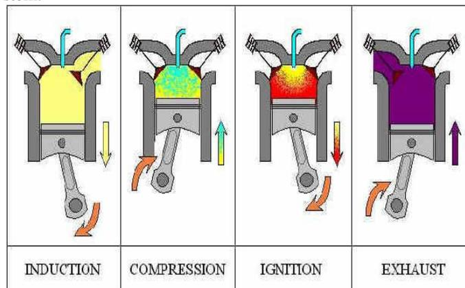
Fig. 3: Diesel Engine Four Stroke Cycle
