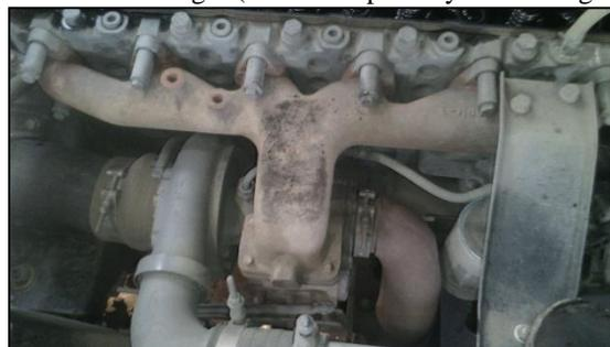
Fig. 8: Single Turbo Arrangement in Dump Trucks
