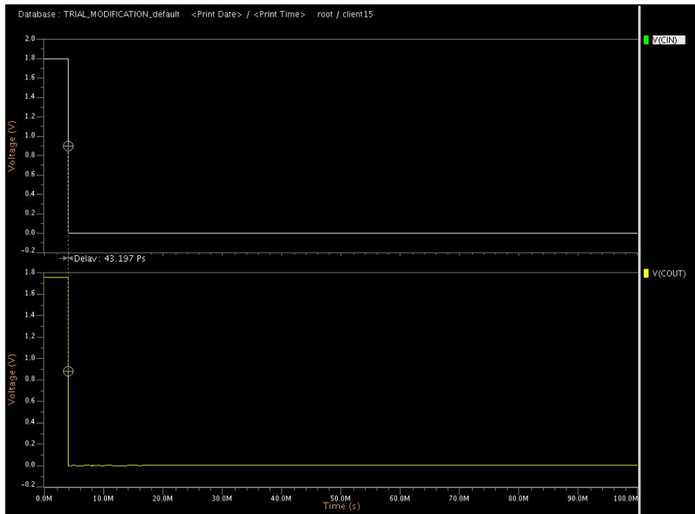
Fig. 8: Simulated Delay Of Proposed Design
