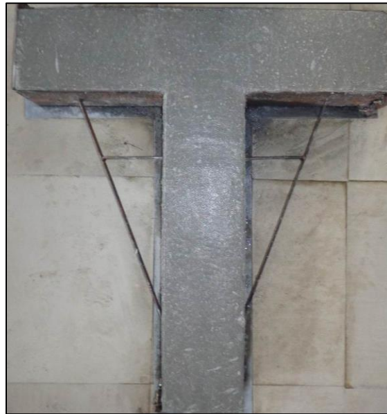
Fig. 2: Beam Column Joint With Specimen
