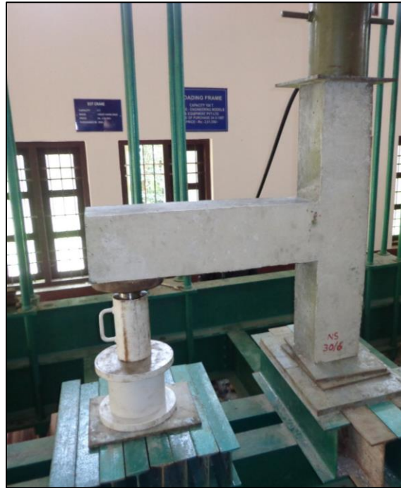
Fig. 3: Beam-Column Joint Placed On Loading Frame For Testing
