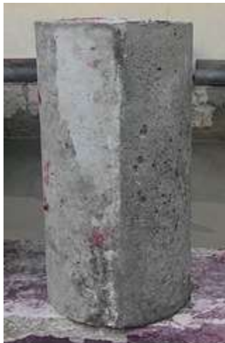
Fig. 4: Split cylinder test full specimen
