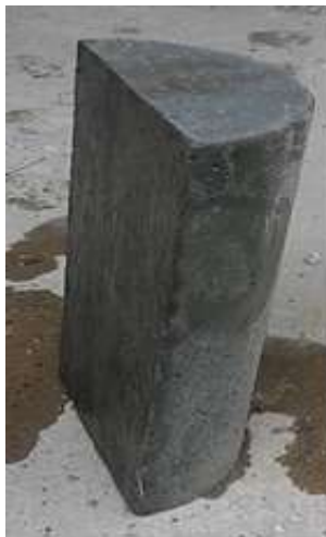
Fig. 3: Split cylinder test substrate portion
