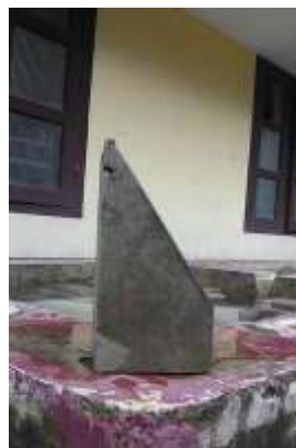
Fig. 1: Slant shear test substrate portion
