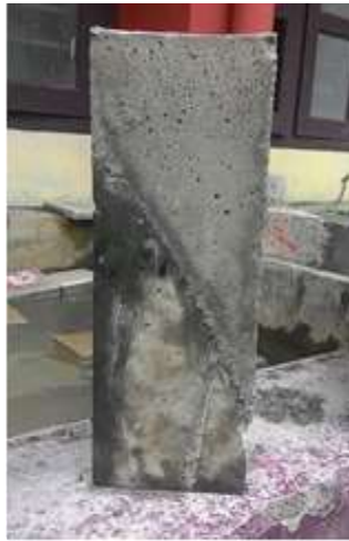
Fig. 2: Slant shear test full specimen
