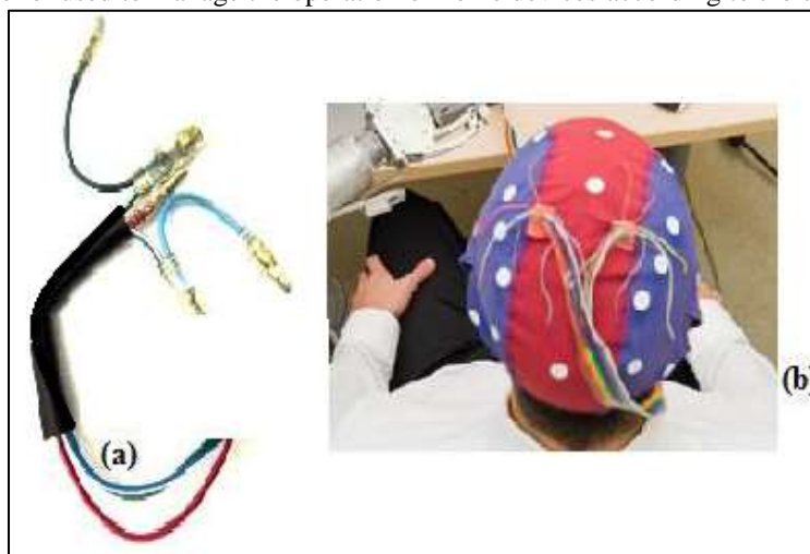
Fig. 1: (a) Mercury tilt switch. (b) a cap that place tilt switch on head.
