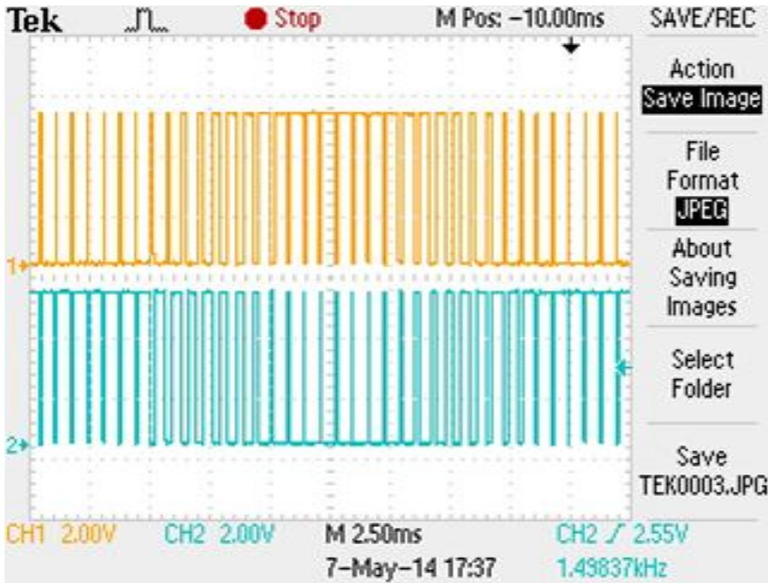
Fig. 13: Generated SPWM Pulses for S1 and S2 Switches of Bridge Inverter.
