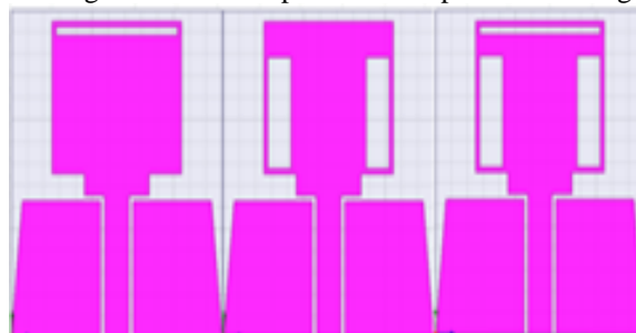
Fig. 3: Design steps of triple slots on primary antenna
