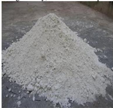
Fig. 1: Hypo Sludge Ash
