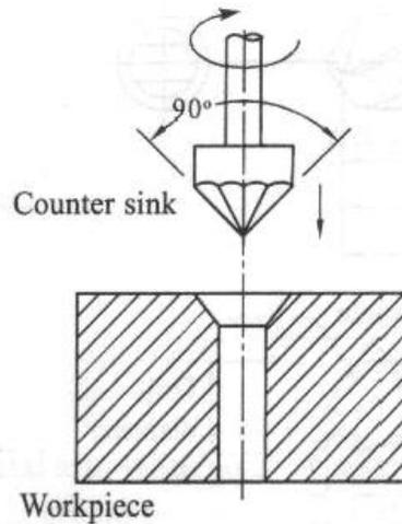
Fig. 3: Counter-sinking
