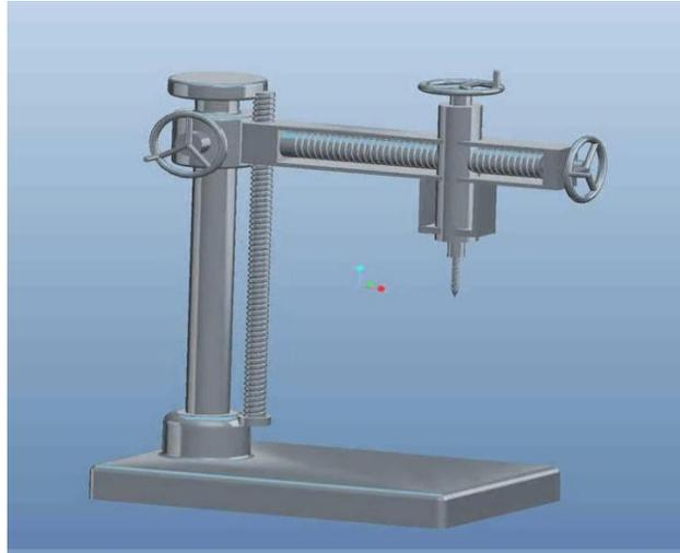
Fig. 8: Design of Universal Micro Radial Drilling Machine On Pro-E
