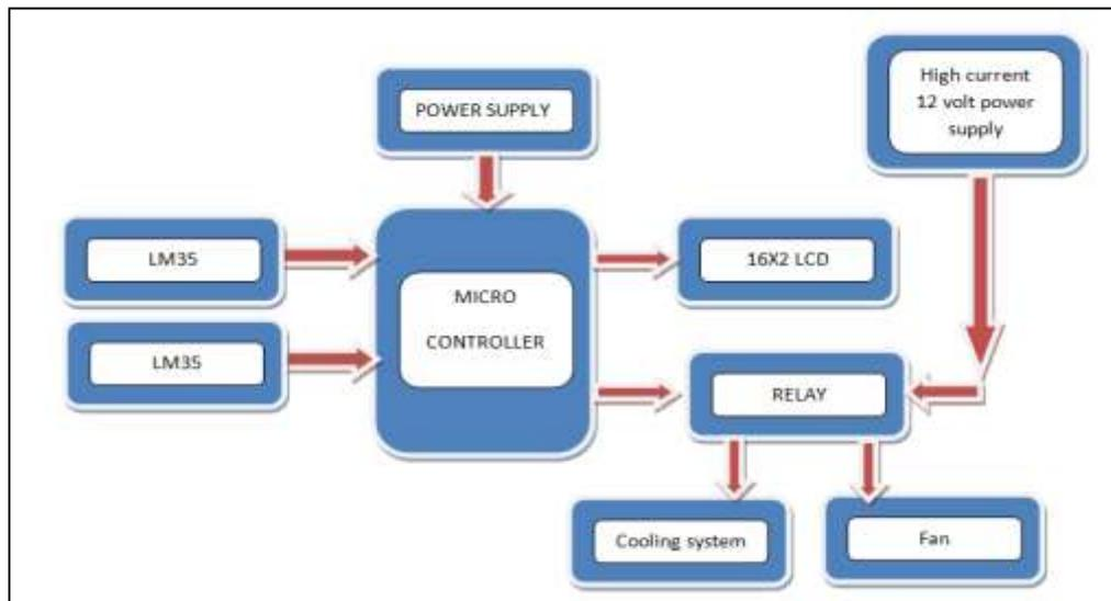
Fig. 4: Block diagram of thermoelectric refrigeration system
