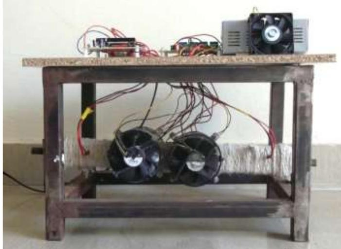
Fig. 2: Front view of experimental set up of thermoelectric refrigeration system
