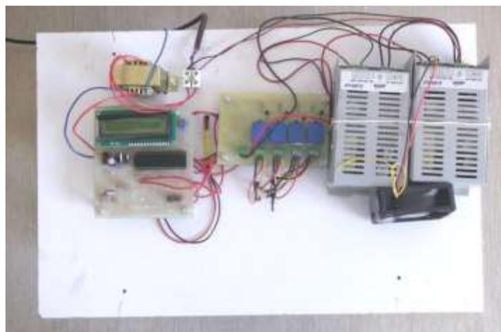
Fig. 3: Top View of experimental set up of thermoelectric refrigeration system
