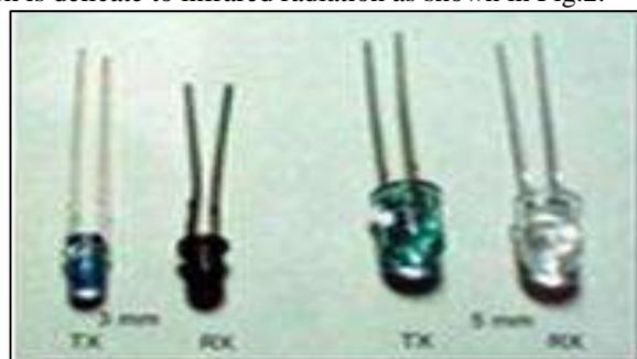
Fig. 2: Images of IR Sensors Transmitter and Receiver
