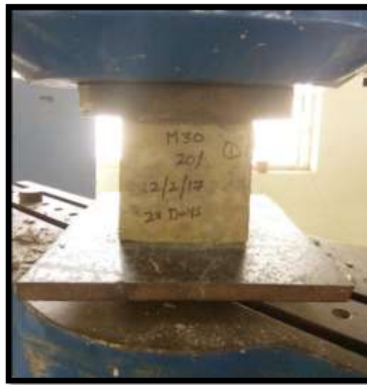
Fig. 1: Compressive strength test
