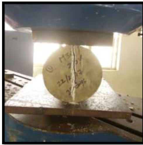
Fig. 4: Split tensile strength test
