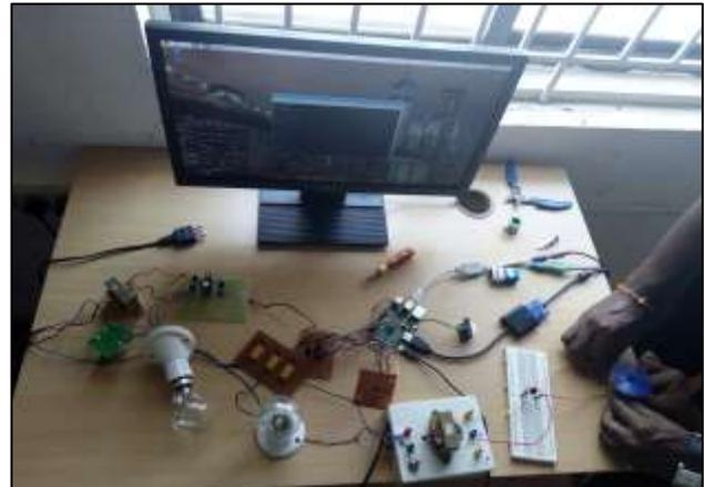
Fig. 8: Controlling Fan by Temperature
