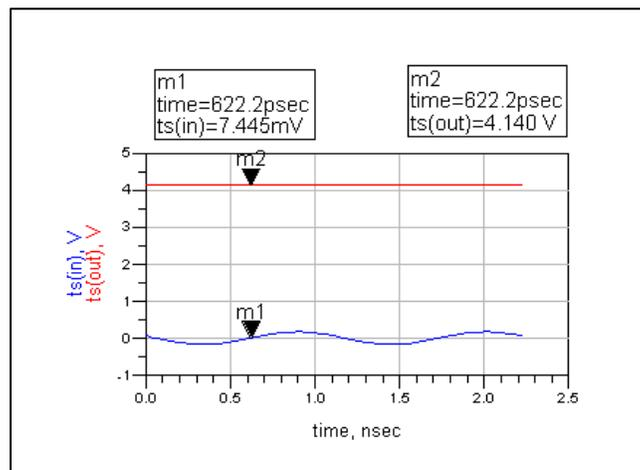
Fig.4.4: Two stage voltage multiplier output
