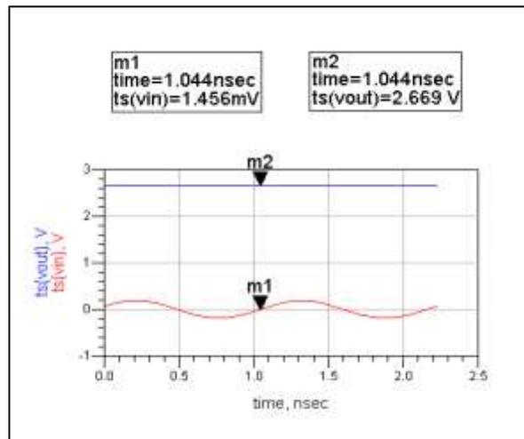
Fig. 4.3: Single stage voltage multiplier output.
