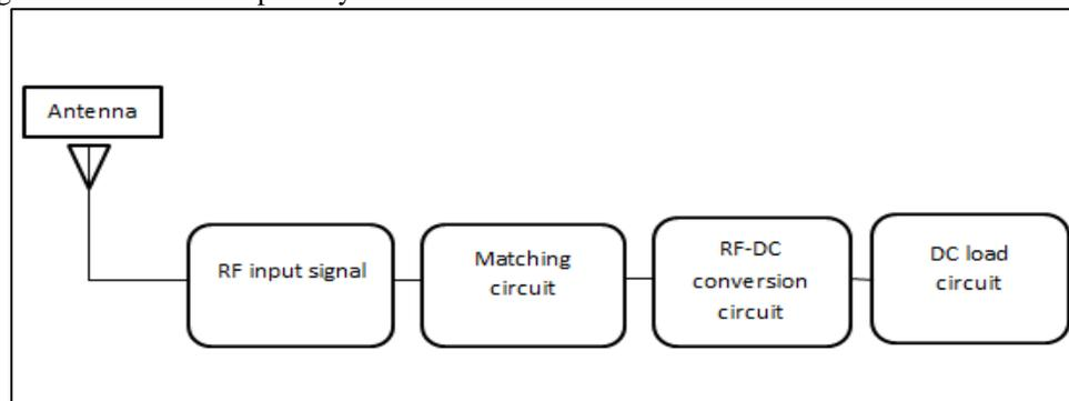
Fig. 1: Block diagram of rectenna
