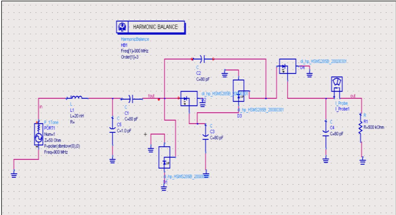
Fig. 3.2: Two stage voltage multiplier
