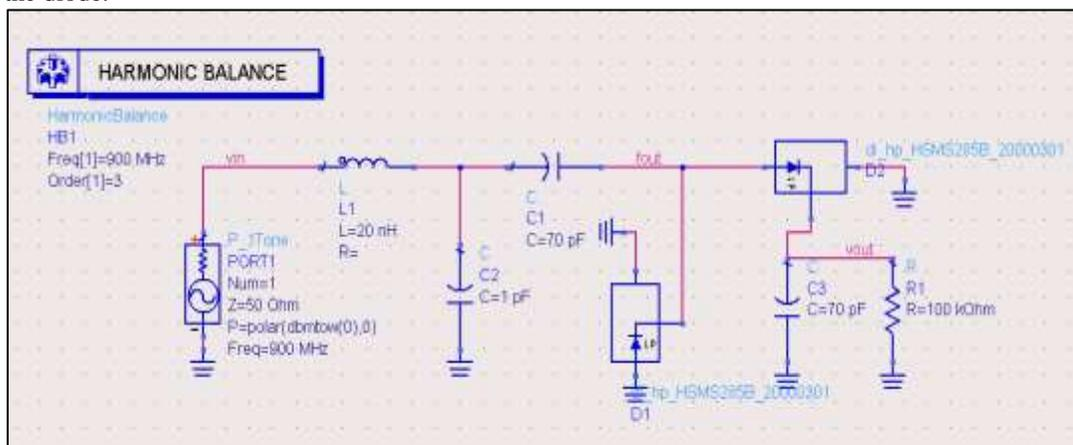
Fig. 3.1: single stage voltage multiplier
