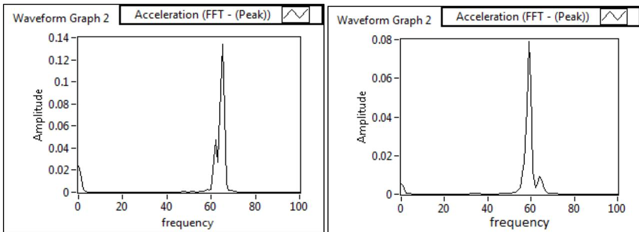
Fig. 2: Amplitude vs frequency graph of normal glass fibre beam
