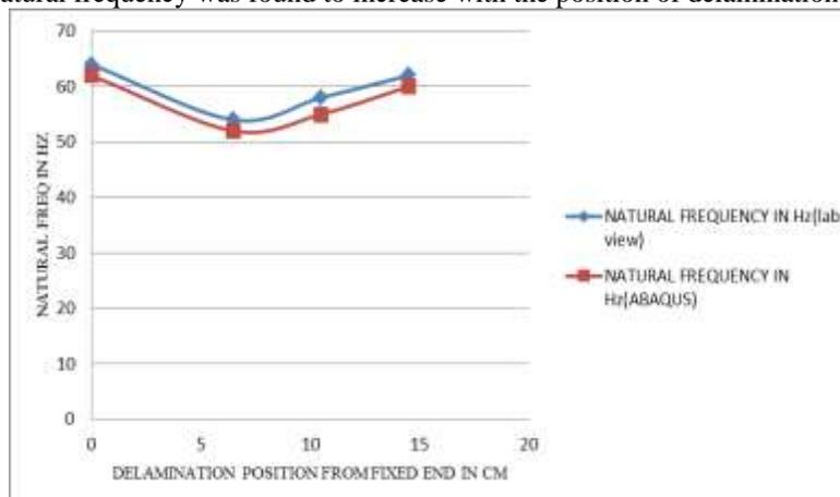
Fig. 11: Natural frequency vs delamination position
