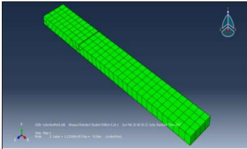
Fig. 10: Abaqus result for delaminated beam at two third length
