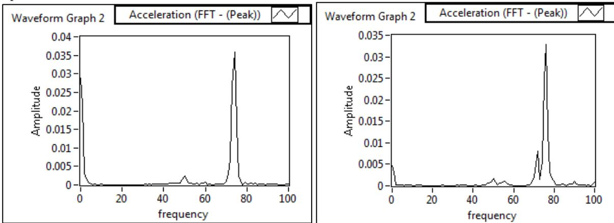
Fig. 1: Amplitude vs frequency graph of steel beam
