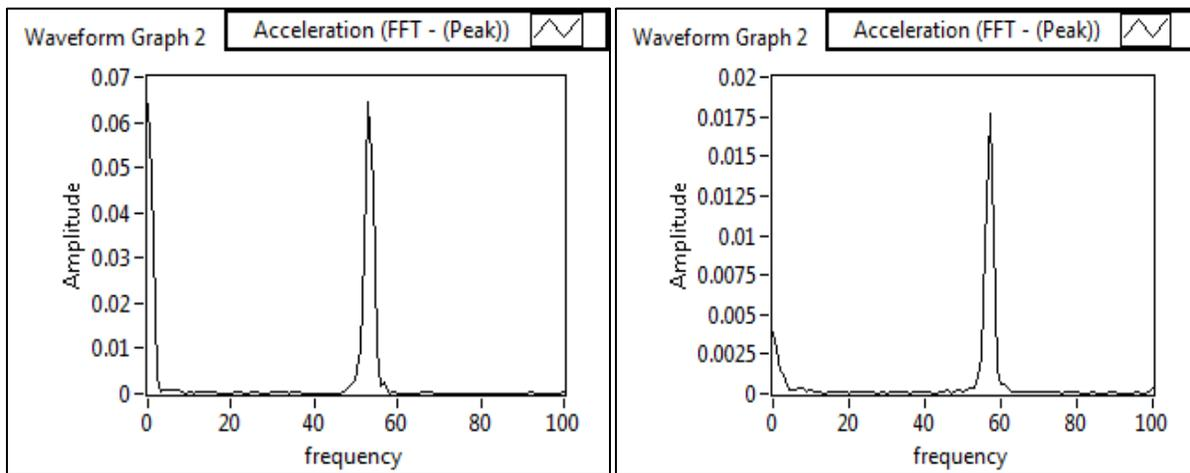
Fig. 5: Amplitude vs frequency graph of delaminated glass fibre beam at two third length
