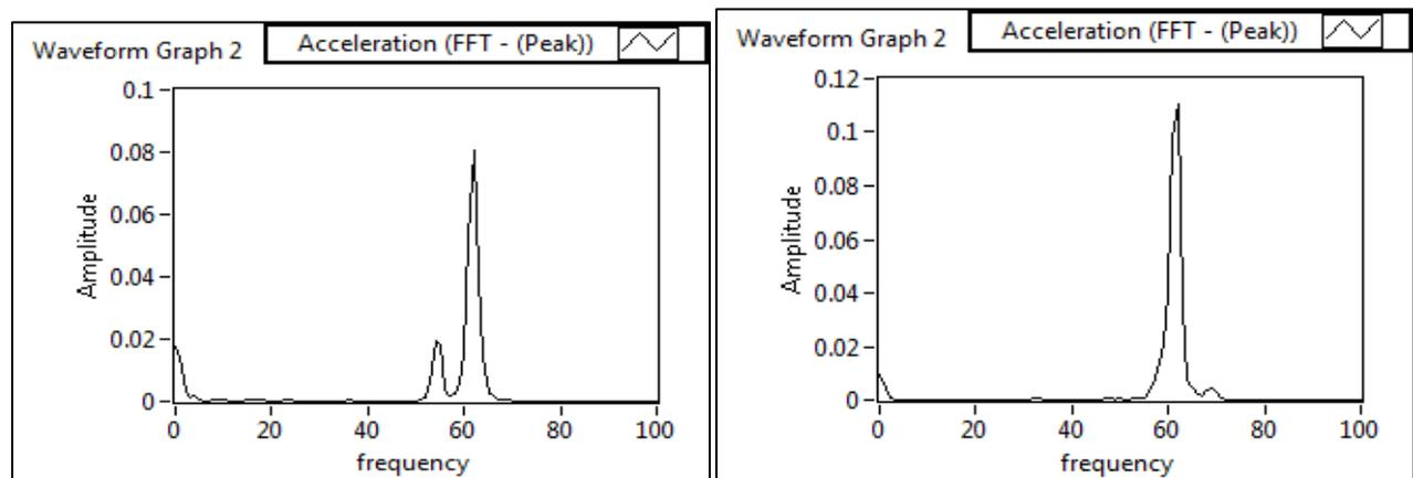
Fig. 3: Amplitude vs frequency graph of delaminated glass fibre beam at one third length
