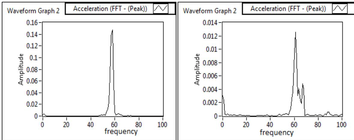
Fig. 4: Amplitude vs frequency graph of delaminated glass fibre beam at half length
