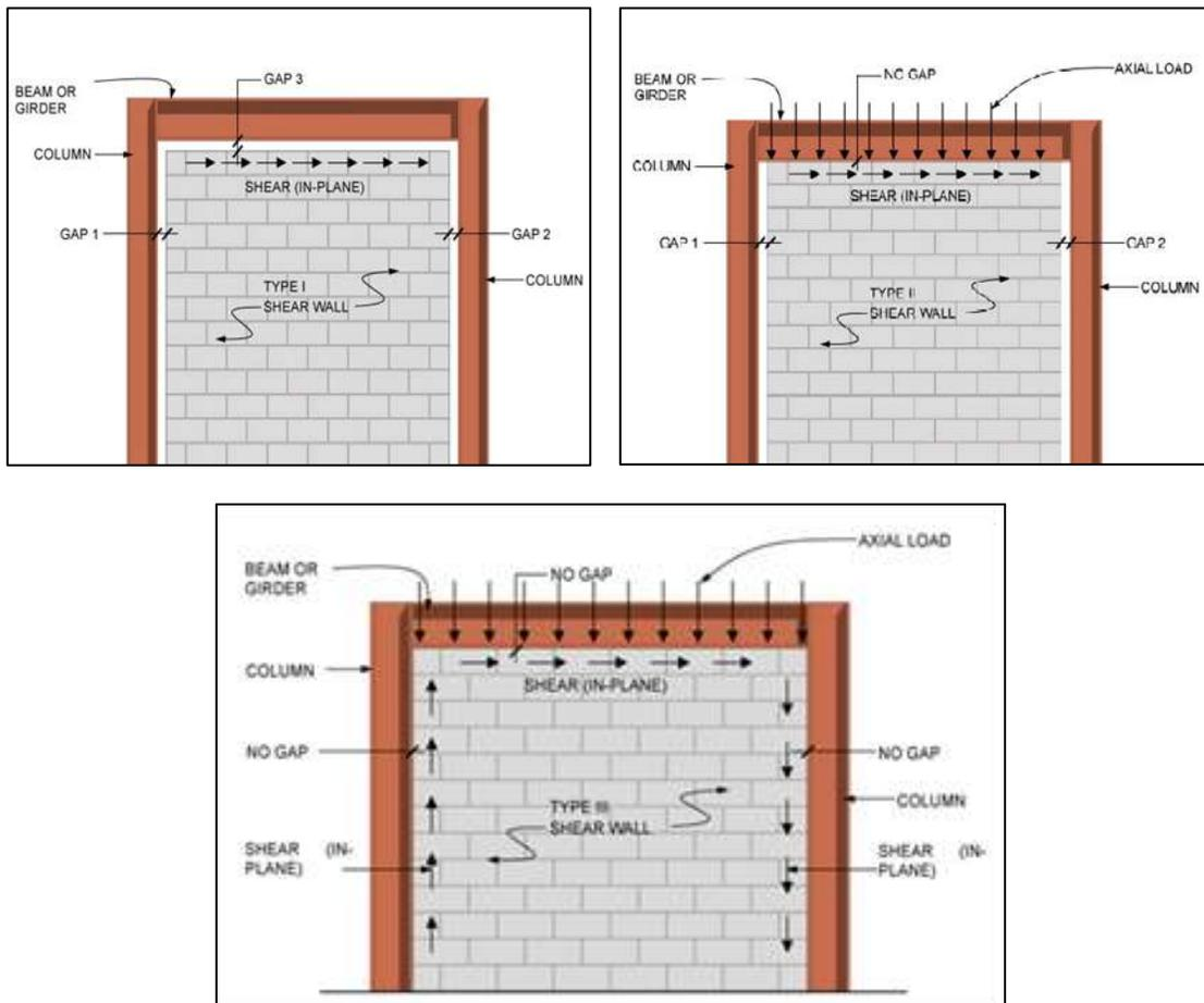
Fig. 1: type I Type II and Type III hybrid walls in clockwise direction respectively [2]
