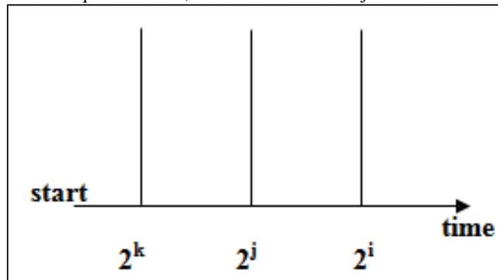
Fig. 4.2: Three nodes with address  $i, j, k$  where  $i > j > k$  with their waiting time.
