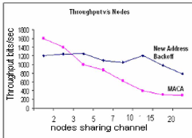
Fig. 5.2: Graph of Throughput vs number of nodes sharing channel
