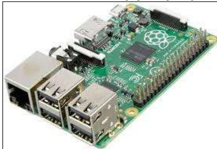
Fig 2: Raspberry Pi 3 model B
