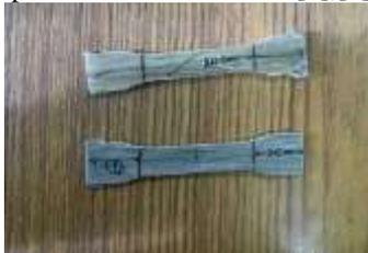
Fig. 1: Specimen For Tensile Test
