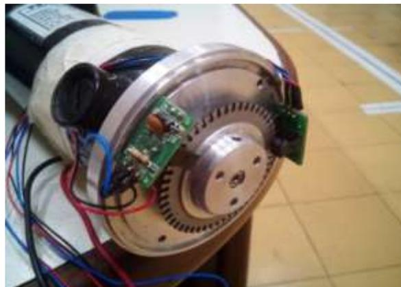
Fig. 3: Photo Interrupter IC's placed on PMDC motor.
