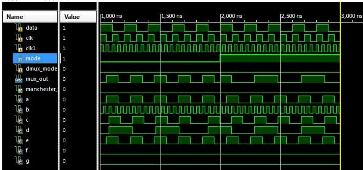
Fig. 5: Simulation result for proposed Manchester and Miller encoder.
