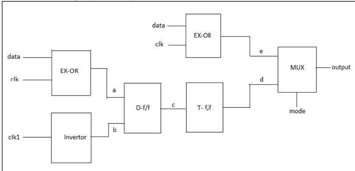
Fig. 3: Prototype Manchester and Miller encoder circuit structure
