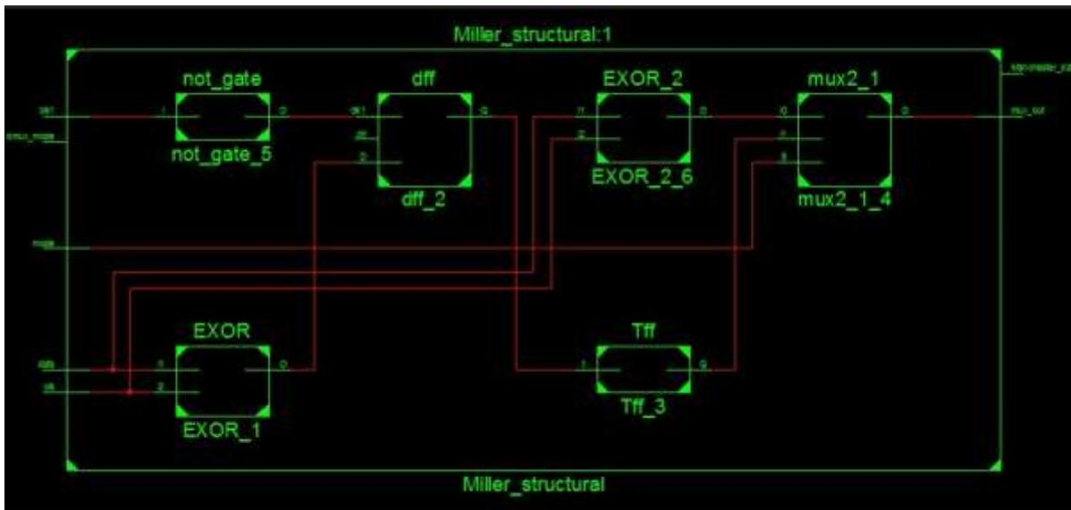
Fig. 4: RTL view of proposed Manchester and Miller encoder
