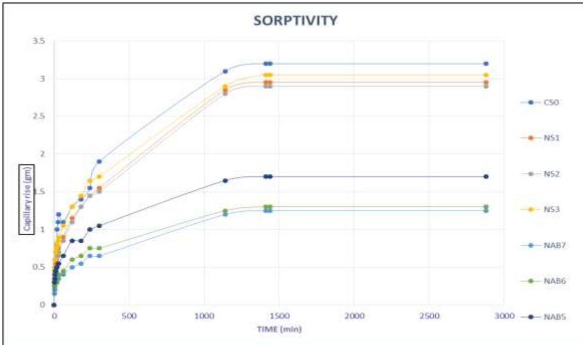
Fig. 5: Comparison of capillary rise for different mix designations
