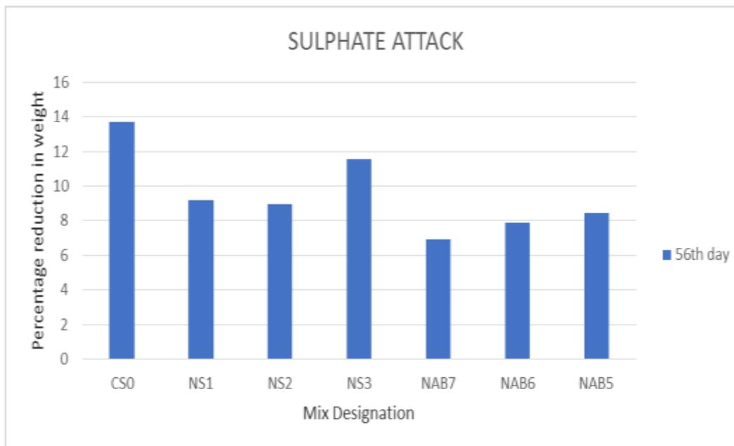
Fig. 2: Comparison of percentage reduction of strength for sulphate attack
