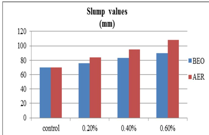
Fig. 1: Variation in slump of different concrete mixes
