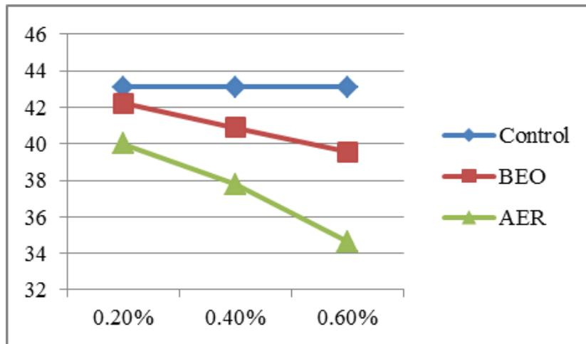
Fig. 4: Variation in 28-days compressive strength (N/mm<sup>2</sup>) Flexural strength
