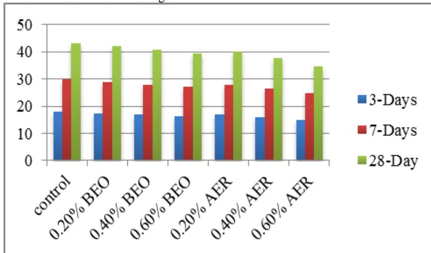
Fig. 3: Variation in compressive strength at different ages (N/mm<sup>2</sup>)
