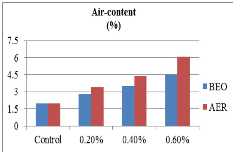
Fig. 2: Variation in air-content of concrete mixes
