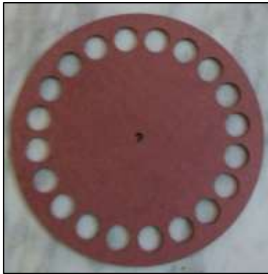
Fig. 4: Magnet disc without magnets
