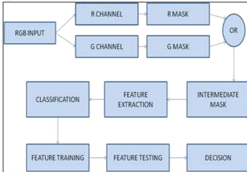
Fig. 3.1: Block Diagram for Maturity of Fruit Detection
