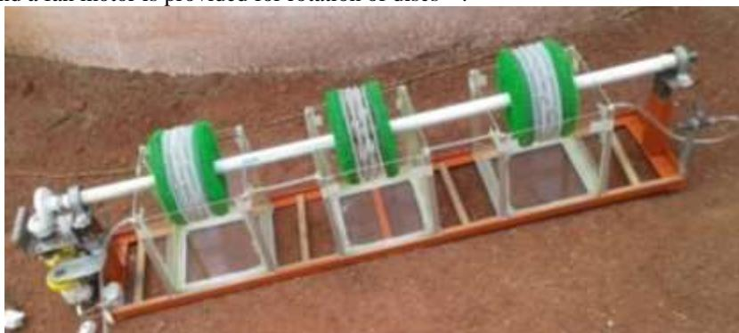
Fig. 2: Fabrication of partially submerged three stage Rotating Biological Contactor (RBC) reactor
