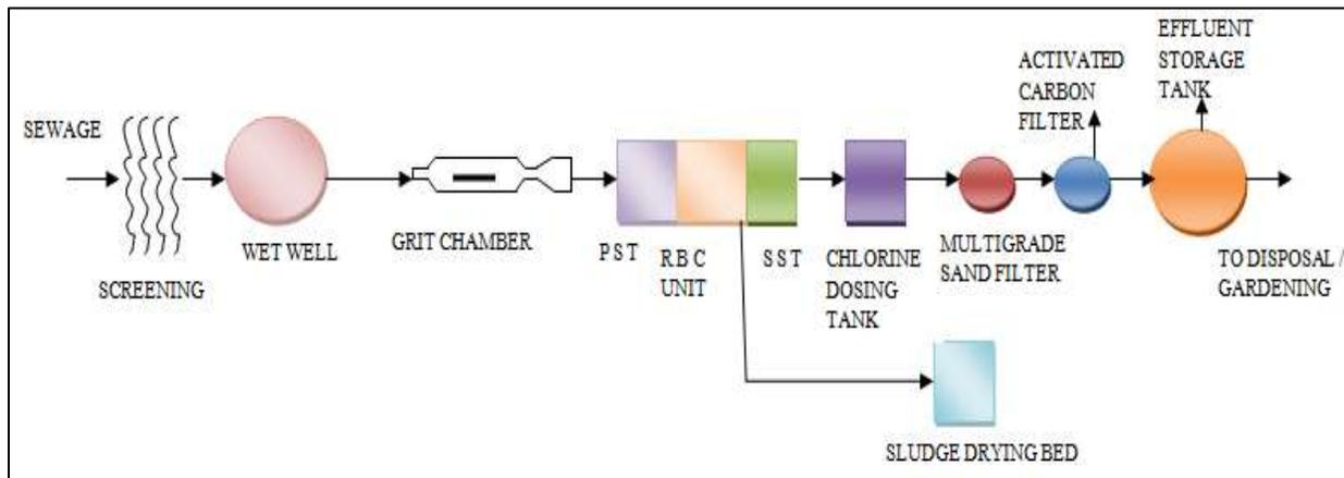
Fig. 1: Flow diagram of Sewage Treatment Plant (STP)
