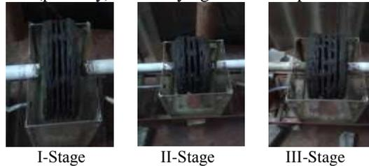
Fig. 3: Development of bio film on the surface of discs in different stages of RBC
