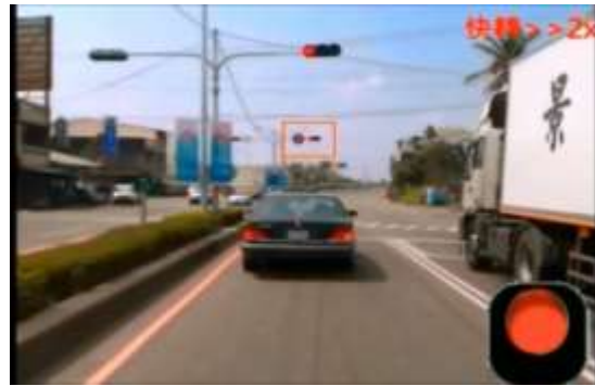
Fig. 1(b): traffic signal light detection
