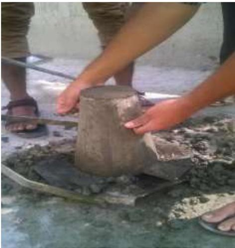
Fig. 1: Slump cone Test showing workability
