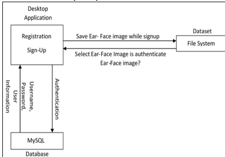
Fig. 4: Architectural Flow of biometric ear and face recognition system
