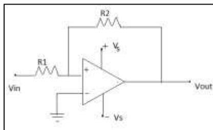
Fig. 2: Schmitt trigger implementation with comparator.
