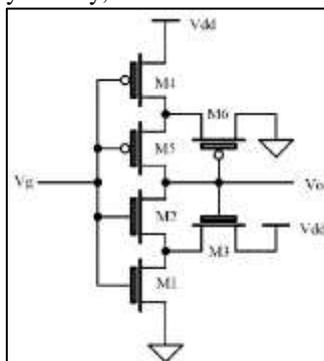
Fig. 3: Low voltage CMOS Schmitt trigger
