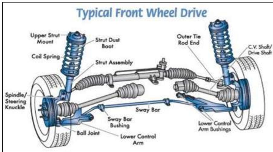
Fig. 3: Front Wheel Suspension system
