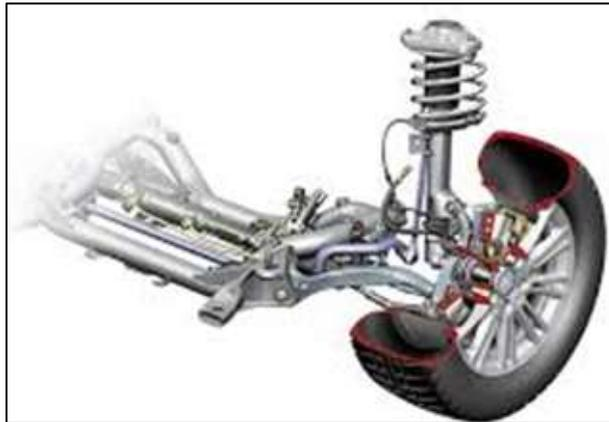
Fig. 1: General Assembly of Suspension System
