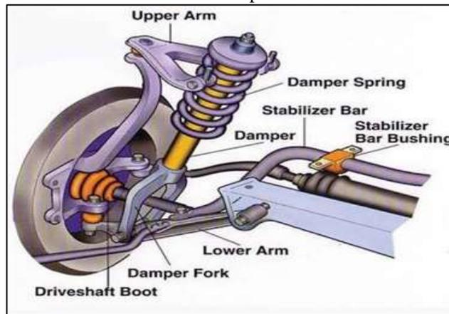
Fig. 2: Various Elements of Suspension System
