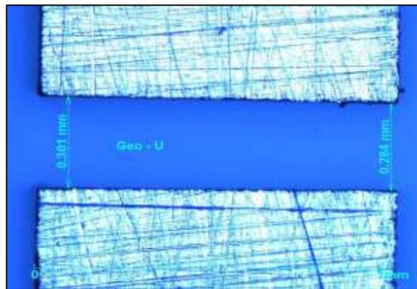
Fig. 1: Throttle geometry “U” in 300 μm thick sheet steel
