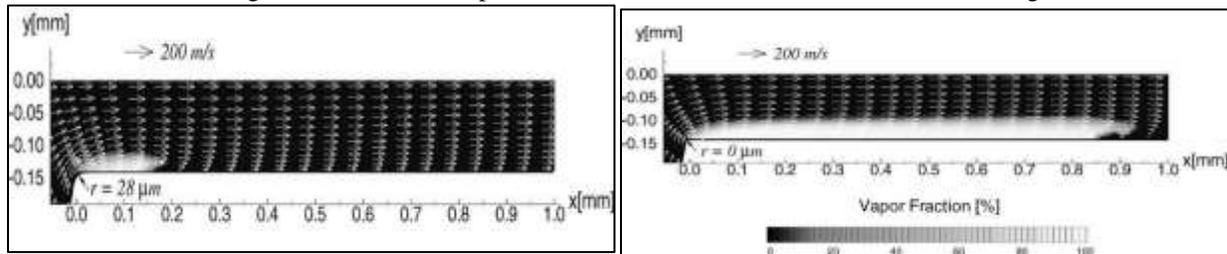
Fig. 3: Computed steady vapour fraction distributions for different tip rounding  $r$ . (For  $P_{in}=80$  bar and  $P_{out}=21$  bar)<sup>[9]</sup>
