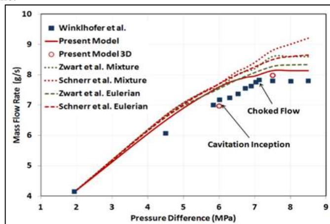
Fig. 4: Comparison of results of various cavitation models [6]
