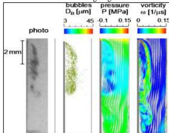
Fig. 2: Observed and calculated cavitation flows ( $V_n = 12.8$  m/s)
