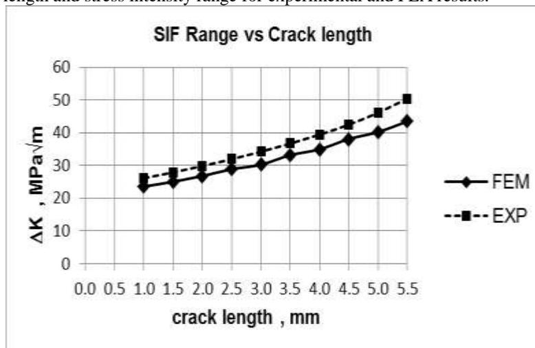
Fig. 7: Characteristic relation between crack length and stress intensity range.
