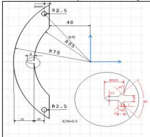
Fig. 1: Specimen geometry
