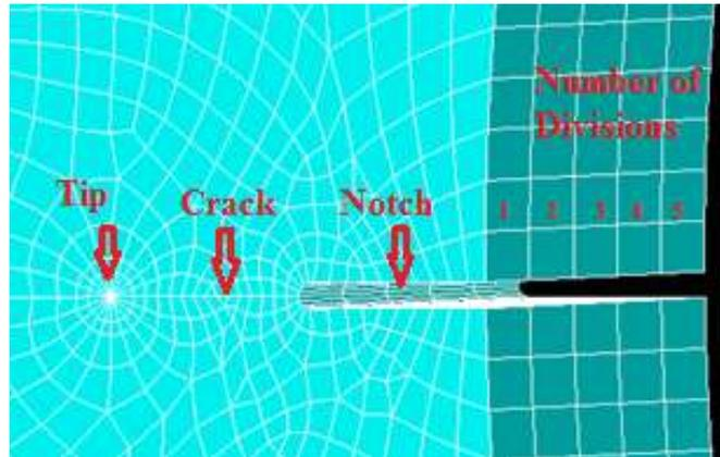
Fig. 6: Finite element mesh with notch and crack
