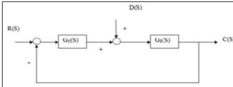
Fig. 7: Block Diagram Of A Typical PID Control System.
