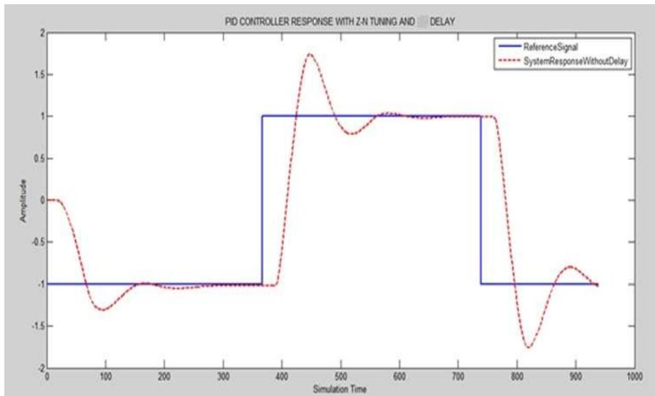
Fig. 9: System response with delay and in presence of PID controller
