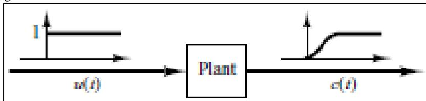
Fig. 4: Unit-Step Response of a Plant
