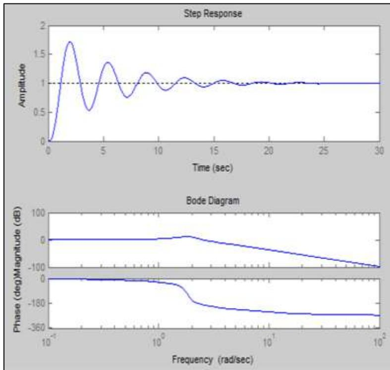
Fig. 11: (a) Output of PID Controller (b) Magnitude and (c) Phase Response at  $K_p = 0.3$  and  $K_i = 1.5$
