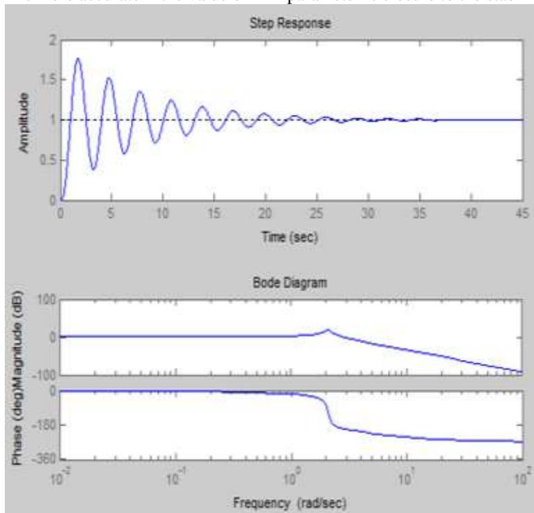
Fig. 10: (a) Output of PID Controller (b) Magnitude and (c) Phase Response at  $K_p = 0.2$  and  $K_i = 2$
