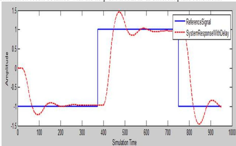
Fig. 8: System response with delay and absence of controller
