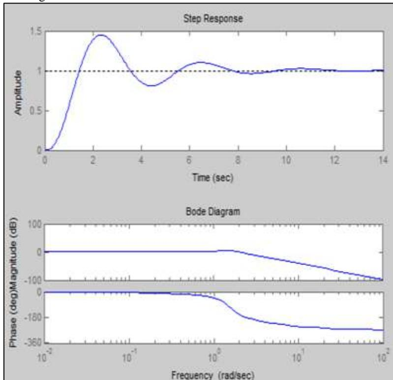
Fig. 12: (a) Output of PID Controller (b) Magnitude and (c) Phase Response at  $K_p = 0.1$  and  $K_i = 1$
