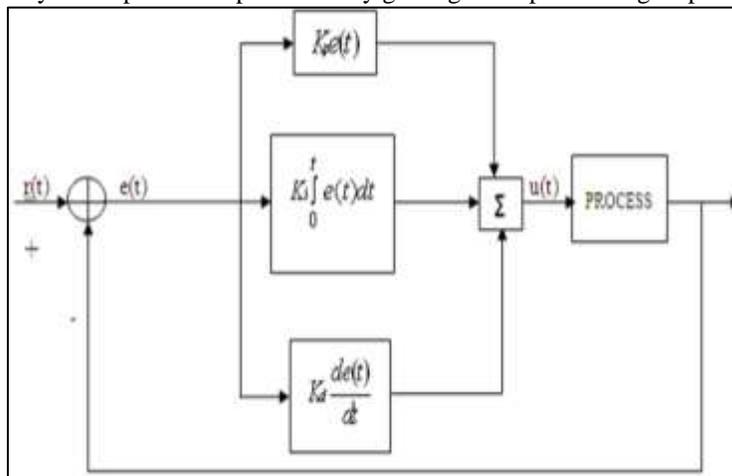
Fig. 3: Proportional- Integral Derivative (PID) Controller Block Diagram
