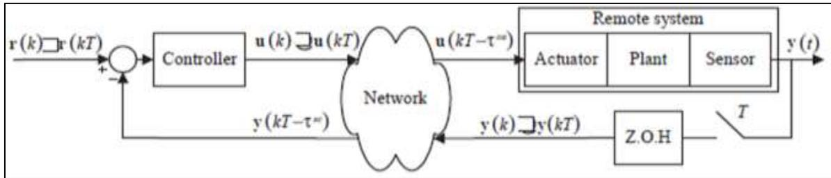
Fig. 2: General NCS Configuration and Network Delays for NCS Formulations
