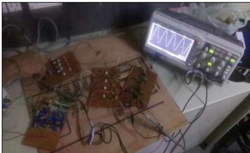
Fig. 17: Testing of AC output of BDHC
