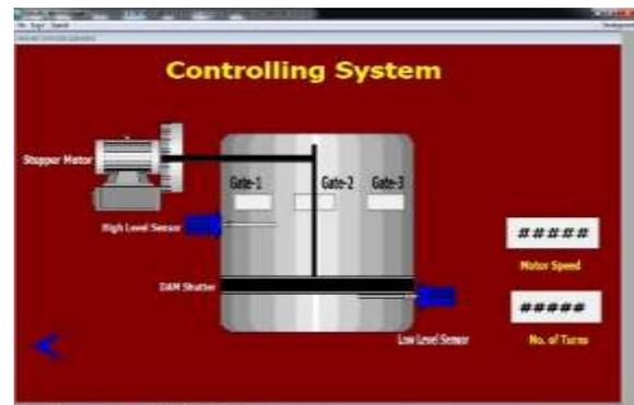
Fig. 6: SCADA design in Intouch Software
