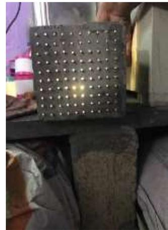
Fig. 3: showing concrete cube with Glued optical fiber
