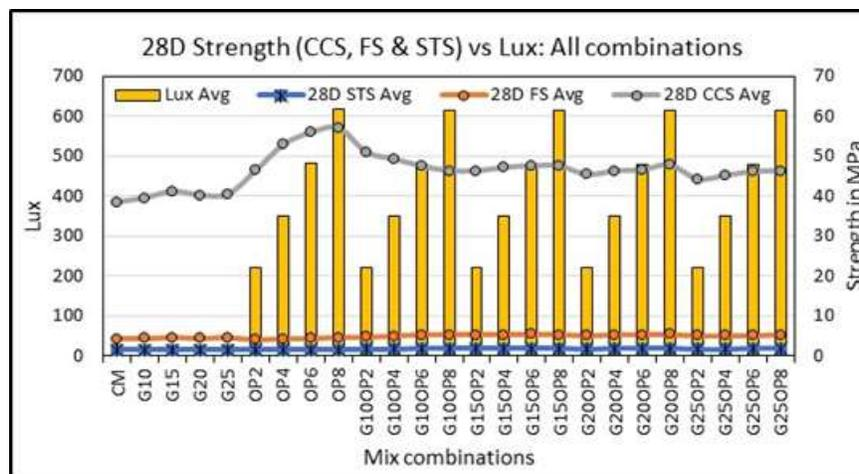
Fig. 7: Light Transmission and Strength comparison
