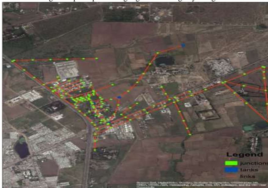
Fig. 8: Georeferencing of Water Distribution Network of Sayajipura Village Using ARCGIS
