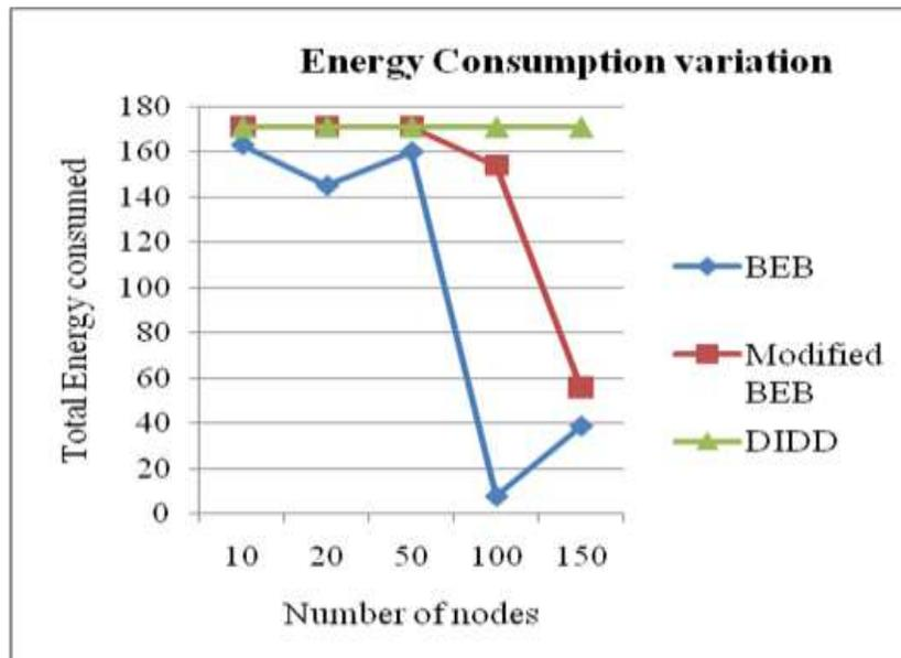
Fig. 13: Graphical Analysis of Total Energy variation for BEB, Modified BEB, DIDD Back off algorithms.
