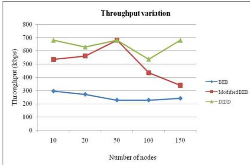
Fig. 10: Graphical Analysis of Throughput variation for BEB, Modified BEB, DIDD Back off algorithms.
