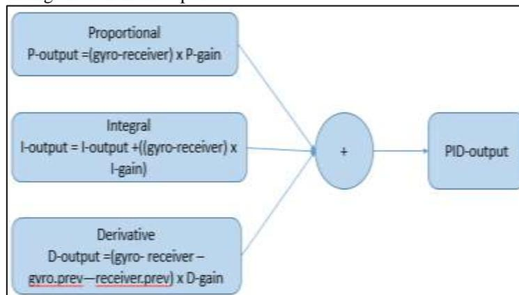
Fig. 3: Block diagram of PID
