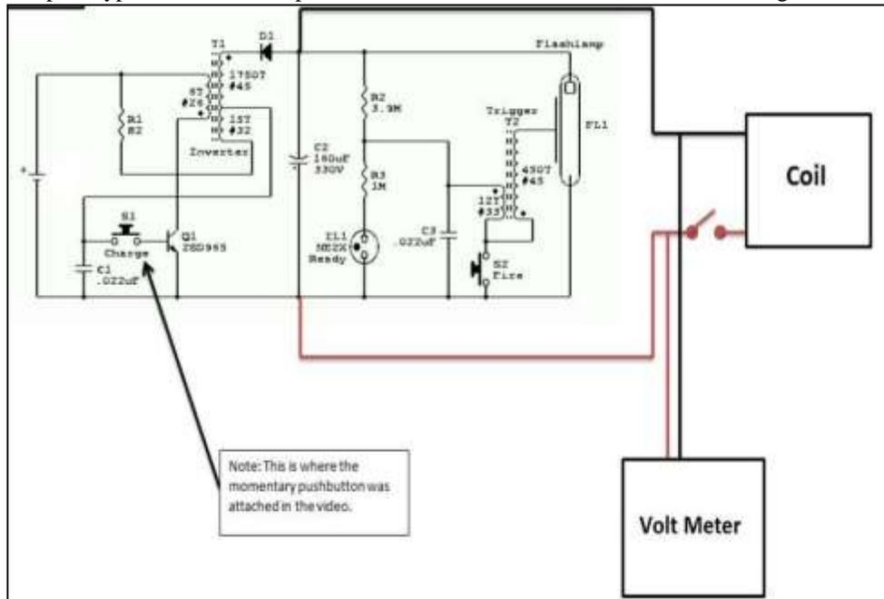
Fig. 4: Schematic Diagram of EMP
