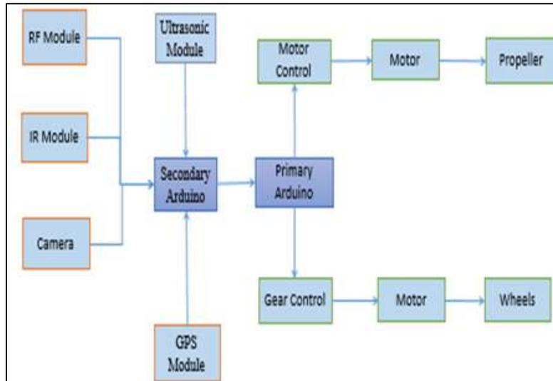
Fig. 2: Block diagram of drone
