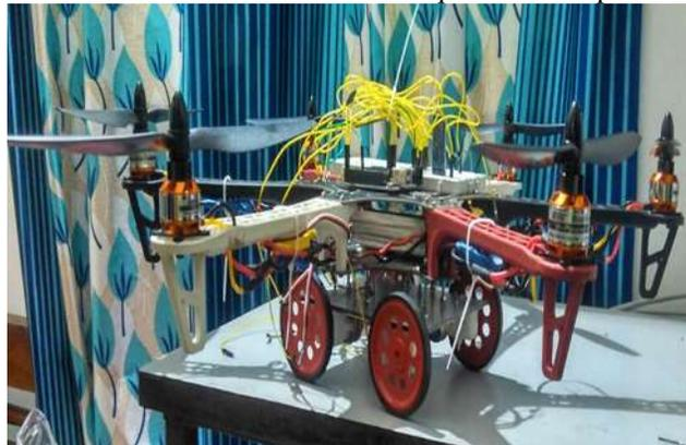
Fig. 1: Drone with rover attached
