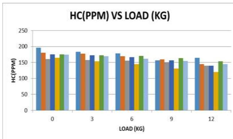
Fig. 5: Variation in HC Emission with Load
