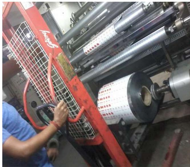
Fig. 19: Proposed method of handling rolls
