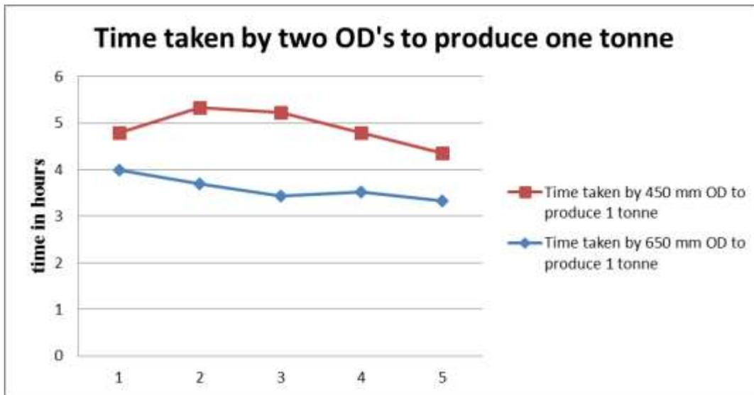
Fig. 16: Improvement in productivity using 650 mm OD
