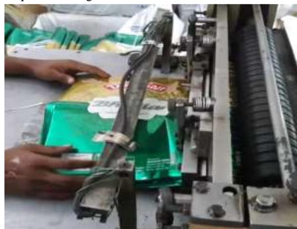
Fig. 6: Pouch Making Machine
