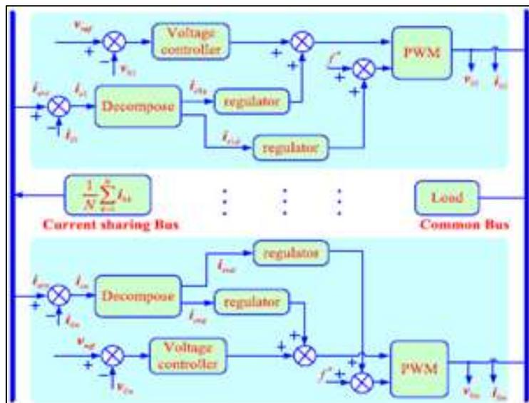
Fig. 2: Control scheme of Distributed Control
