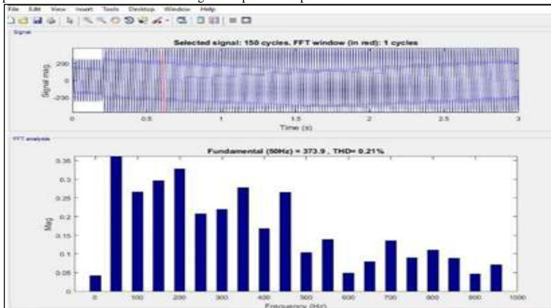
Fig. 11: Showing the harmonics level in reactive power control technique
