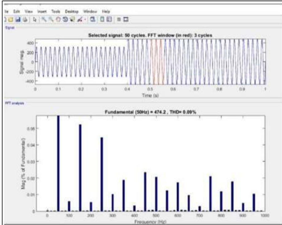
Fig. 8: Showing harmonics level in Droop control method
