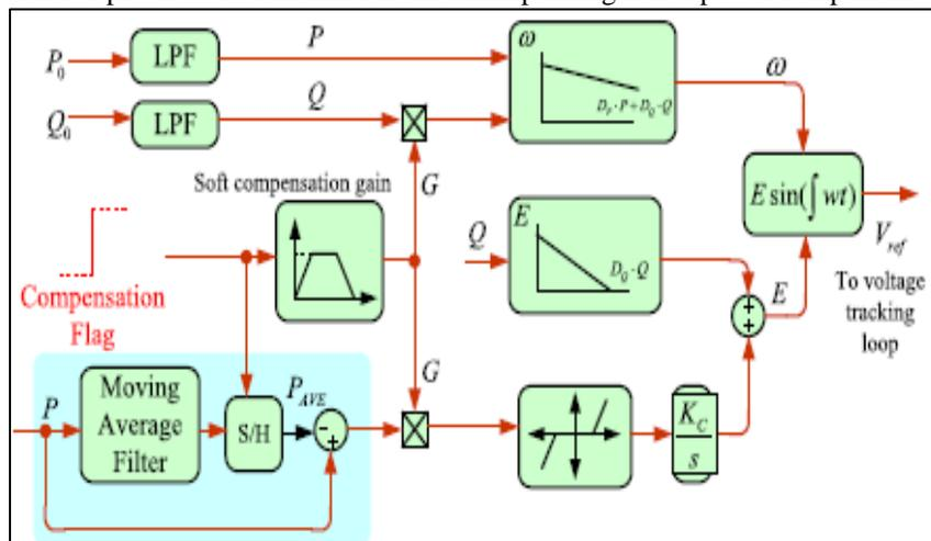
Fig. 4: Control scheme of reactive power control
