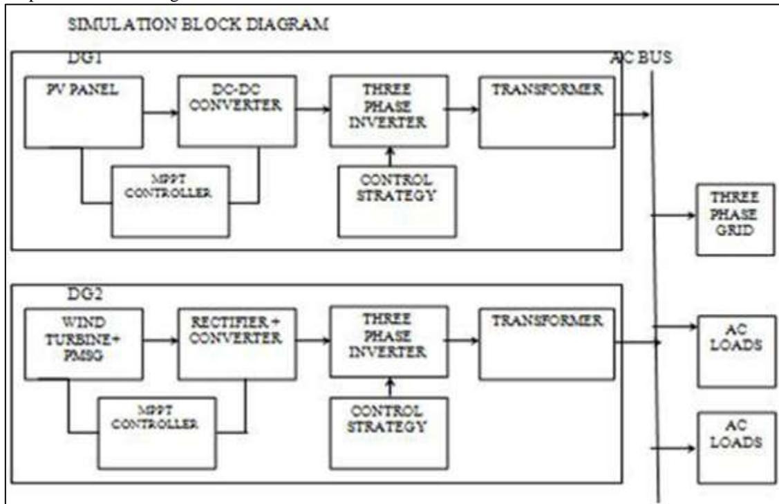
Fig. 5: Simulation Block Diagram
