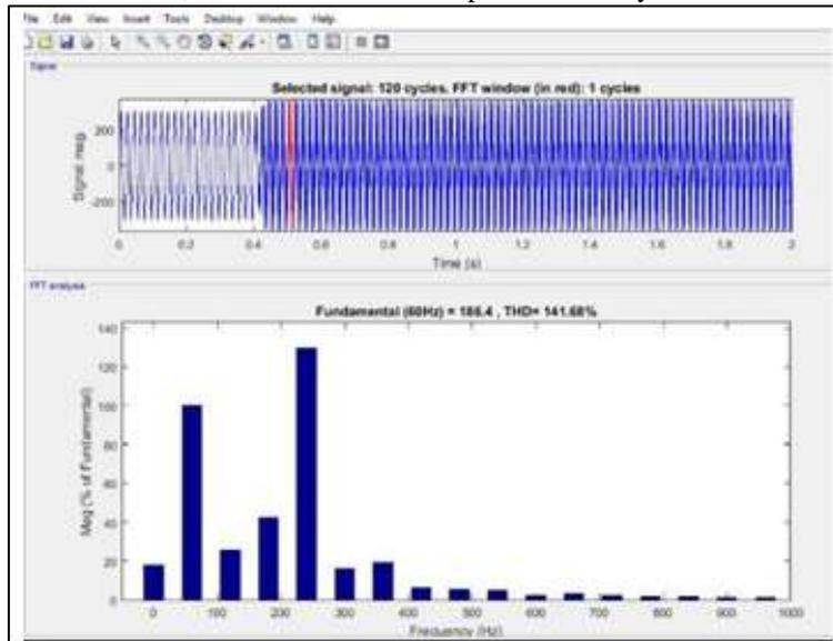
Fig. 7: Showing harmonics level in Distributed control method
