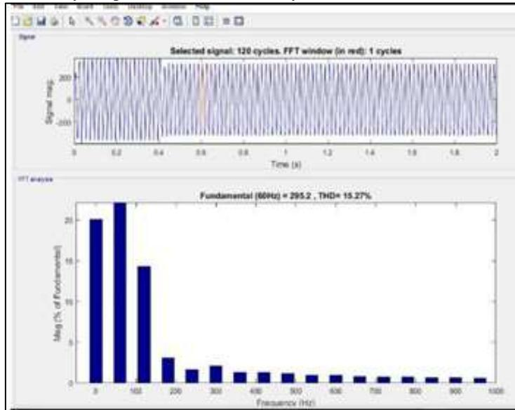
Fig. 6: Showing harmonics level in concentrated control method
