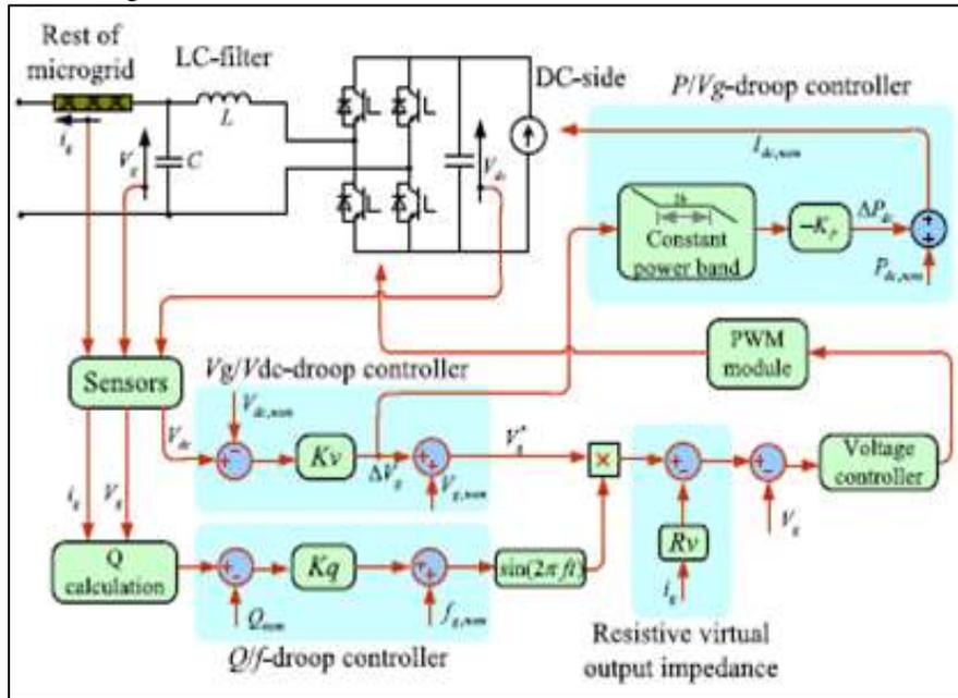
Fig. 3: Control scheme of droop Control with constant power band
