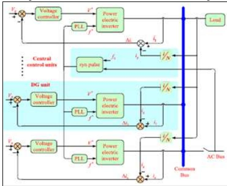
Fig. 1: Control scheme of Concentrated Control
