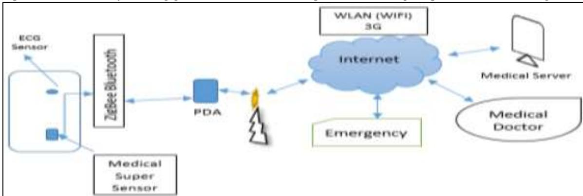
Fig. 5: BSNs: A method to screen Heart Rate [21]
