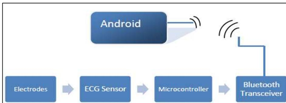
Fig.6. WBAN for heart attack detection [21]
