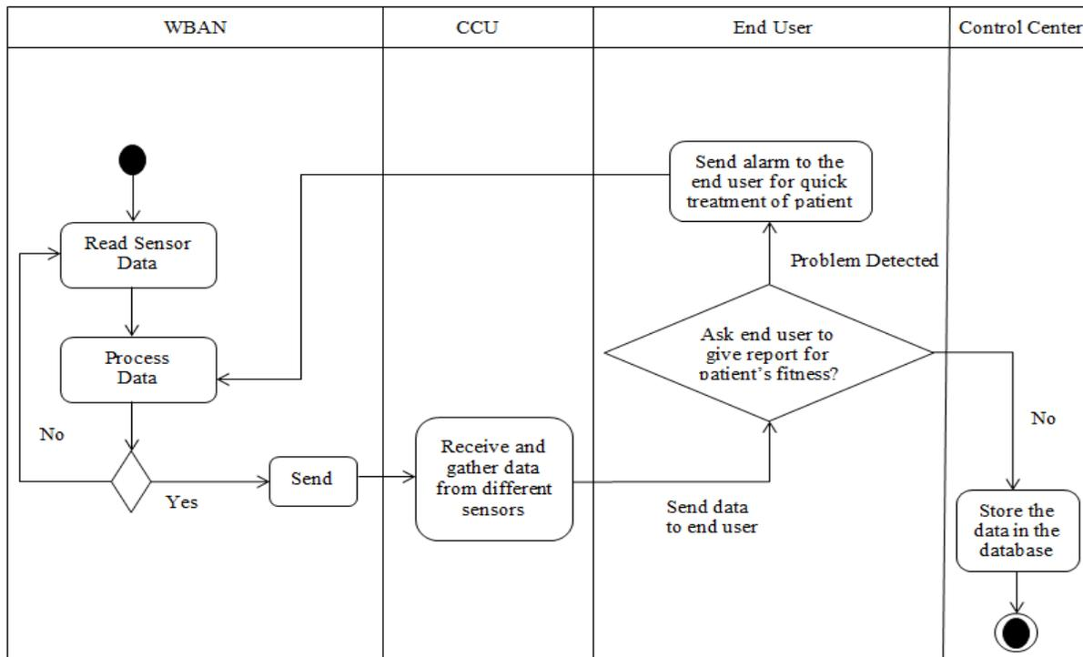
Fig. 2: Activity diagram of WBAN Architecture
