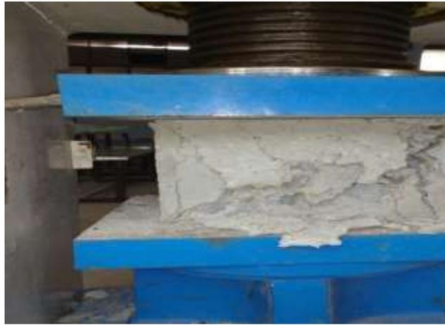
Fig. 1: The compression testing arrangement for concrete cubes.
