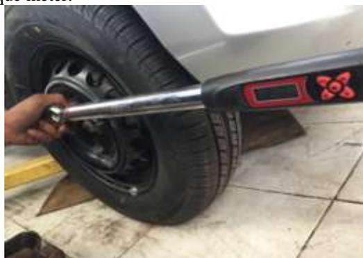
Fig. 9: Find Out Torque for Opening a Nut
